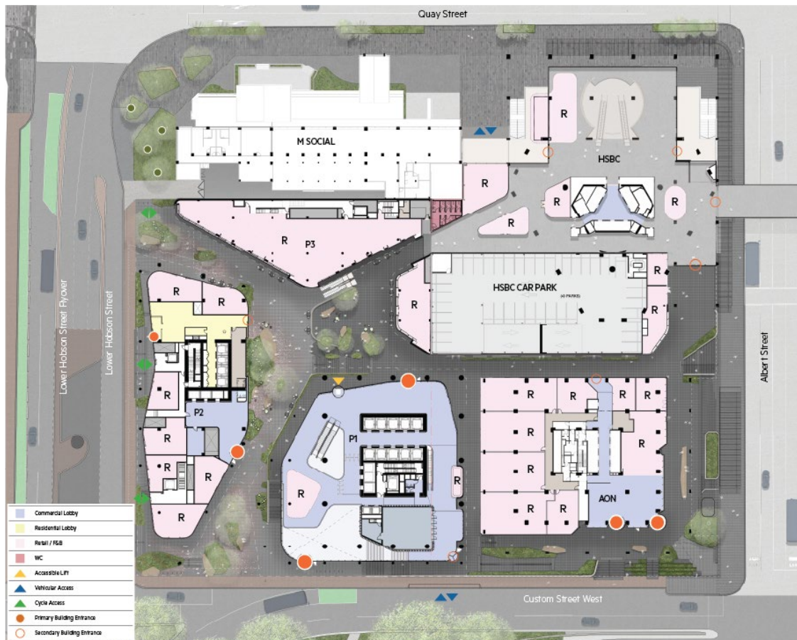
Figure 4.33 Hybrid plan showing lower ground floor under T2 at left (Level 00) and upper ground floor (Level 01) with entries and indicative retail tenancies.
