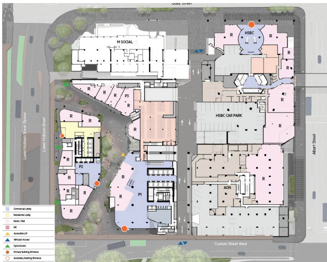
Figure 4.7 Lower ground floor plan (Level 00) with activities and entries shown with a red marker.
